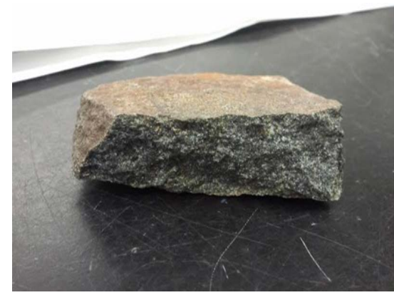
Diabase with coarser grains than sample above showing different rates of cooling throughout the sill. Dark pyroxene and lighter plagioclase feldspar grains visible.
